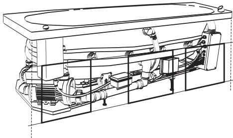
**!** For the operation of the whirl system it is absolutely necessary that air can circulate underneath the pool. An air grid with a ventilation cross section of at least 80 cm<sup>2</sup> has to be provided in the blower area.
