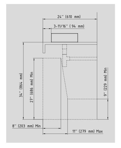
Model meets ADA guidelines when installed according to recommended ADA installation.
