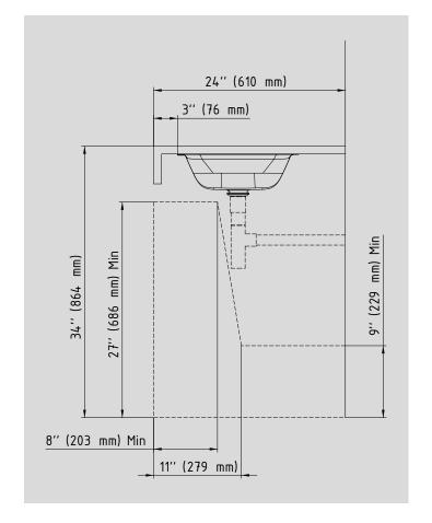
Models meet ADA guidelines when installed according to recommended ADA installation.
